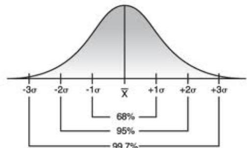
This picture shows a normal distribution and the percentages of data that fall within one, two and three standard deviations ( $\pm \sigma, \pm 2\sigma, \text{ and } \pm 3\sigma$ ) from the mean ( $\bar{x}$ )
